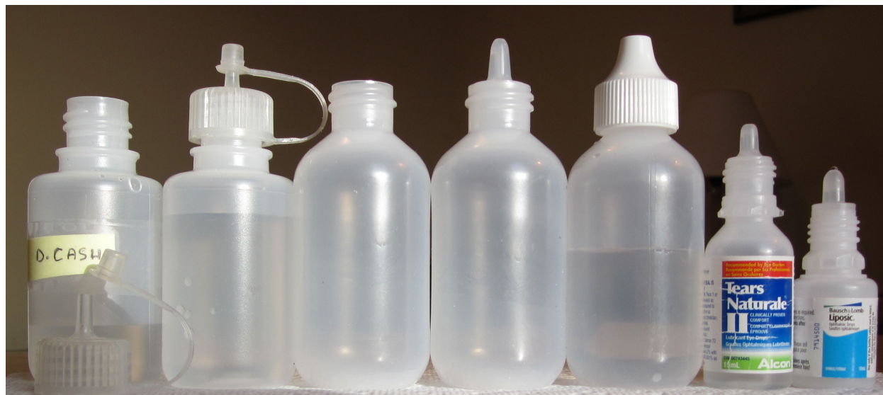
Photograph: Polymer Drop-Dispensing Squeeze-Bottles (Credit D. Cash 2012) Left: Two 60 mL Nalgene Bottles: One-Piece Integrated Tip and Cap (cost: about $ 72 per dozen) Centre: Three 60 mL Wheaton Bottles: Inner Snap-Out Tip and Outer Closed Cap (cost: about $ 30 per dozen) Right: 15 mL and 10 mL Eye-Drop Bottles: Inner Snap-Out Tips Shown (cost: free eye-drop dispenser empties)
