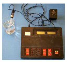
Microprocessor-Controlled Digital pH Meter (Hanna Instruments HI8417)
